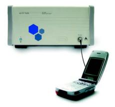
**Off-air** With an off-air connection, the RF socket of the tester is connected connection to Willtek's Antenna Coupler. This makes testing easy and fast. The mobile transmits via the antenna. No further test adapters are needed. The coupling loss depends on factors such as orientation. distance and frequency. To a certain extent, this can be compensated with a coupling loss table.
